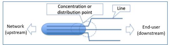
Figure 3: Illustration of a distribution or concentration point <u>without</u> traffic aggregation
