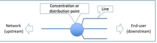
Figure 4: Illustration of a distribution or concentration point <u>with</u> traffic aggregation
