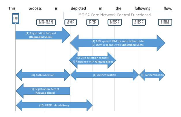
How the traffic originated in the UE is steered over the proper network slice?
