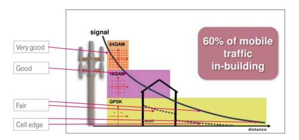
The further away a terminal is from the base station, the more radio resources it occupies in order to receive/transport the same amount of data. This effect effectively reduces the average available capacity per end-user on the air interface.
