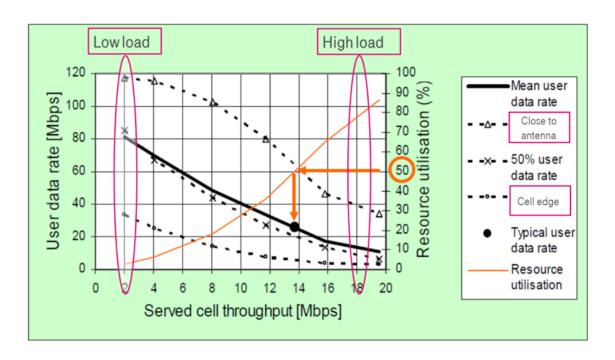
Due to the increased interference levels when network usage increases, the total available air interface capacity will decrease, resulting in an even more reduced average available capacity per user.
