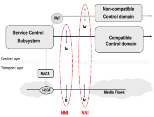
I-BGF: Interconnection Border Gateway Function IWF: InterWorking Function RACS: Resource and Admission Control Subsystem
