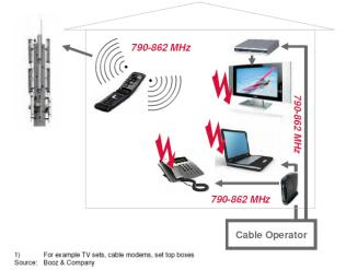
Tests in Germany, Austria and the UK have been carried out that indicate that new mobile broadband services (LTE) are likely to cause interference within customer premises and to customer equipment such as set top boxes, modems, TV sets, flat screens, game consoles... This interference could negatively affect the customer experience with a multitude of UHF receivers.
