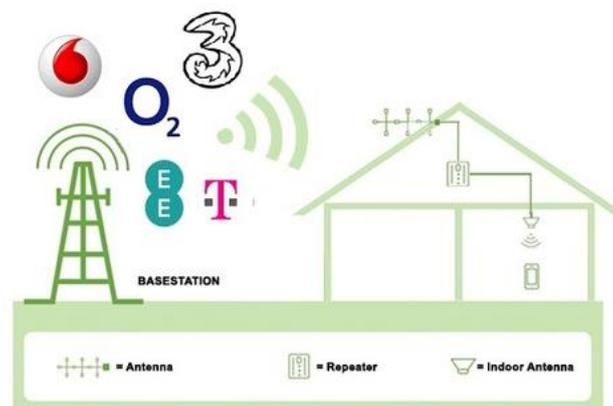
Figure 4 - off the air mobile repeater<sup>17</sup>
