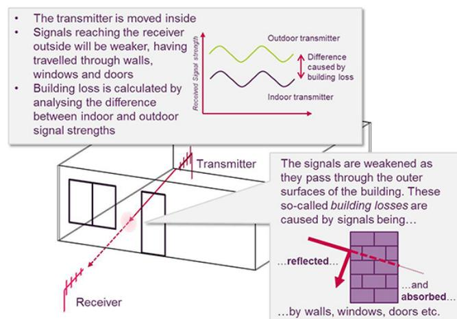
**Figure 2 – Measuring the effects of construction materials on indoor coverage<sup>9</sup>**
