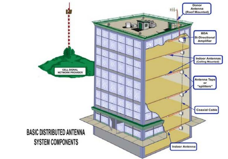
Figure 6 - DAS system components<sup>20</sup>
