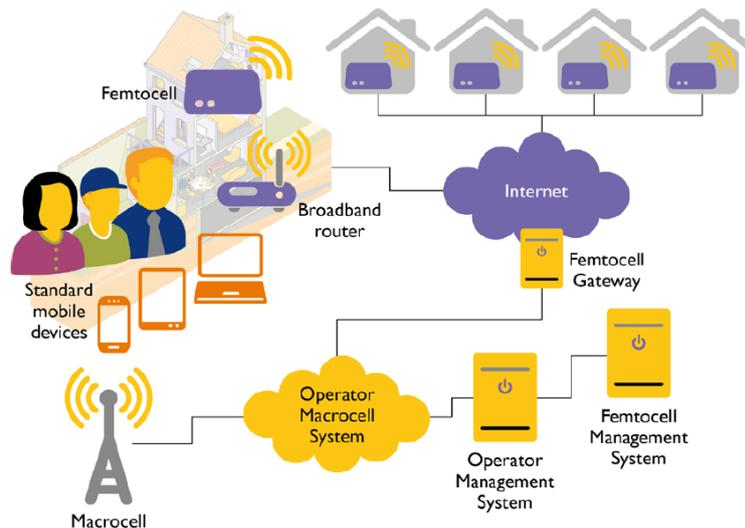
**Figure 5 - Typical Femtocell Deployment Scenario<sup>19</sup>**
